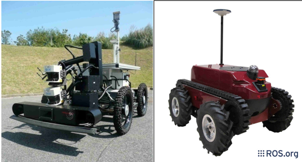
Figure 18: Ground based inspection robots (2) – RobuCARTT and GUARDIAN robot
