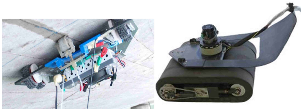
Figure 15: Climbing robots using vacuum adhesion mechanism
